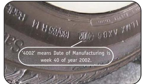
Vehicle tyres have a 4-year validity period from their Date of Manufacture (DOM). Thereafter, the tyre expires and may burst whilst in use. How to find out whether your tyre validity has expired? Check for a stamp '4002' as shown in picture above : The first two numbers '40' indicates the week of the year in which it has been manufactured. The last two numbers '02' represent the year of manufacture. '2699' this shows that the tyre is made in the 26th week of 1999.
