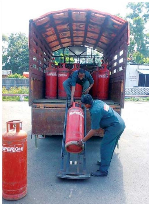
Normally filled and empty cylinders are loaded/unloaded manually from packed cylinders vehicle at plants, franchisee godowns and customer premises by crews. Often it is observed that standard practices of safe handling of cylinders are not followed by crews hence cylinder body, footing, VP ring get damaged during loading/unloading where activity is not being done under supervision.
